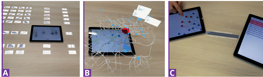
Fig. 6.4.: Three of the use cases presented in MARVIS. In (A), we show additional cells of a SPLOM around the tablet. In (B), the map presented on the display gets extended in AR, also displaying the previously opened Details-on-Demand. In (C), a link between the logically connected tablets is showing, highlighting the number of selected and in-view-port nodes.
