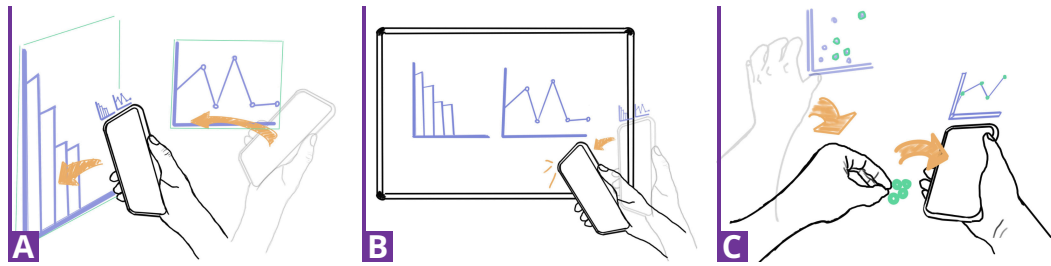
Fig. 6.8.: Three illustrations presenting different envisioned features of the AR Authoring system. (A) shows how a user can collect visualizations via a fishnet metaphor, which can be later on (B) placed on a surface in the immediate environment via tapping the corner of the device on the surface. (C) shows how a filter can be applied to a new visualization by using a selection in another visualization.
