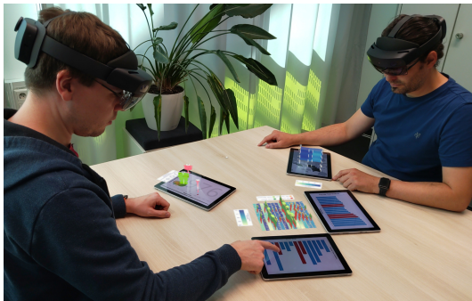
Fig. 6.2.: The prototype system and HUI based on MARVIS. The system can present additional AR information around, above, and between the tablets.
